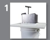
Set up the Gel Cutting Device on the Cutting Board placed over a bucket or storage container.
