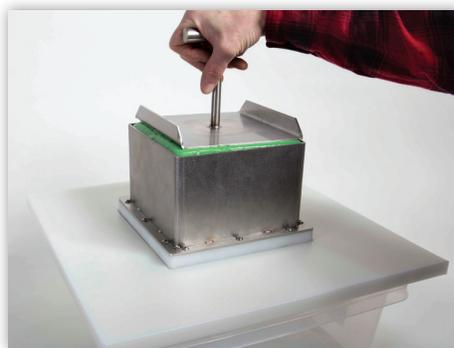
**4** With the Gel Cutting Device plunger, push the gel squares through the blade assembly.
